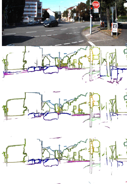
Fig. 1: From top to bottom: DFF (ResNet-50), DFF (MobileNetV2), FENet (ours). Semantic edge maps on KITTI dataset are produced by the network trained on Cityscapes dataset without any finetuning. Our real-time network shows competitive performances compared to existing methods.
